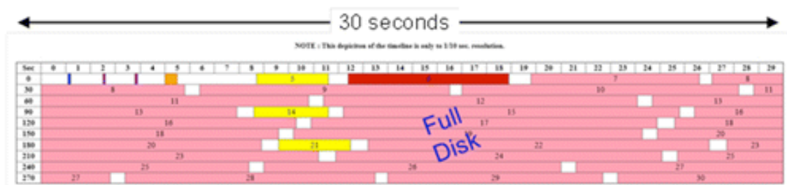
Figure 5: ABI Continuous Full Disk (scan mode 4) timeline diagram. This timeline covers 5 min. Colors same as Figure 4. There are no CONUS or mesoscale scenes in this timeline.
